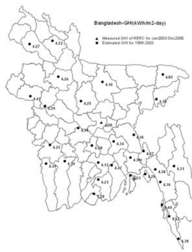
Figure 3: Annual Measured and Estimated GHI at RERC and BMD stations
