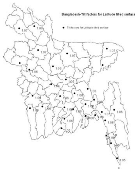
Figure 27: Annual Tilt factors for Latitude tilted surface for all BMD stations
